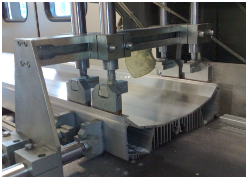
EXAMPLE PHOTO: CUTTING ALUMINIUM PROFILES EVEN OF LARGE DIMENSIONS
