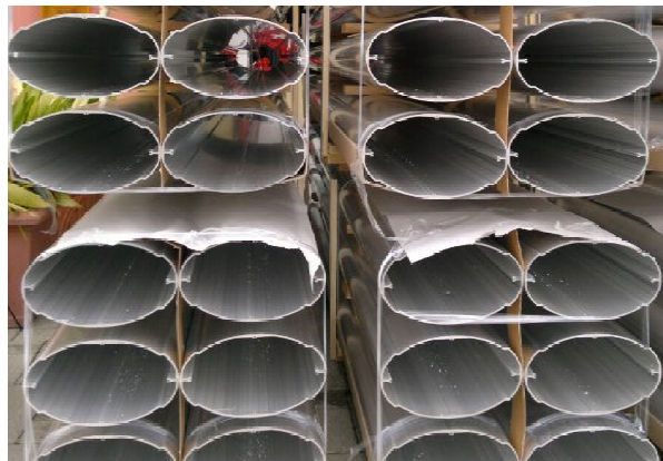
EXAMPLE PHOTO: ALUMINUM EXTRUDED PARTS FOR LIGHTING BODIES
