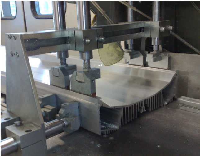
EXAMPLE PHOTO: CUTTING TO SIZE OPERATIONS ARE CARRIED OUT ON ALUMINUM PROFILES
