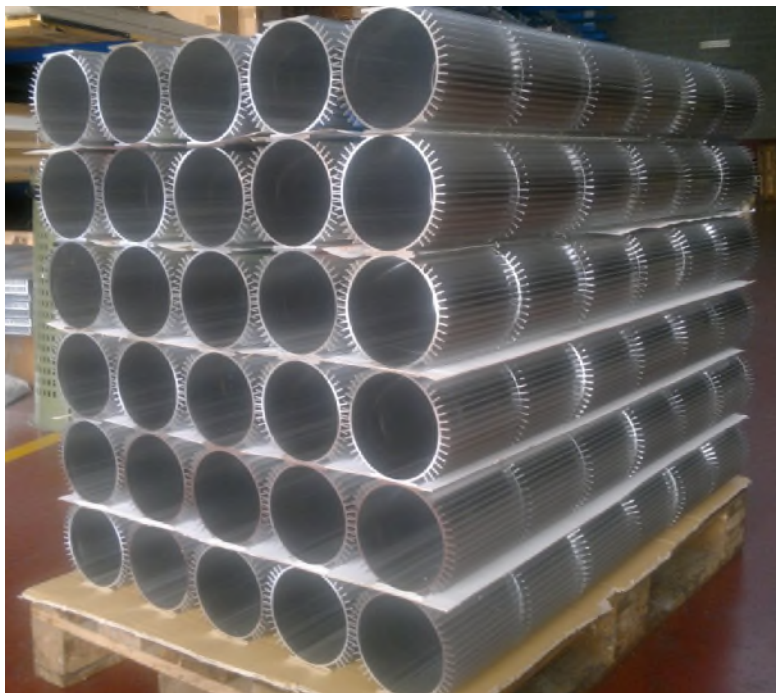
EXAMPLE PHOTO: EXTRUDED ALUMINUM PROFILES FOR ELECTRIC MOTOR CASINGS
